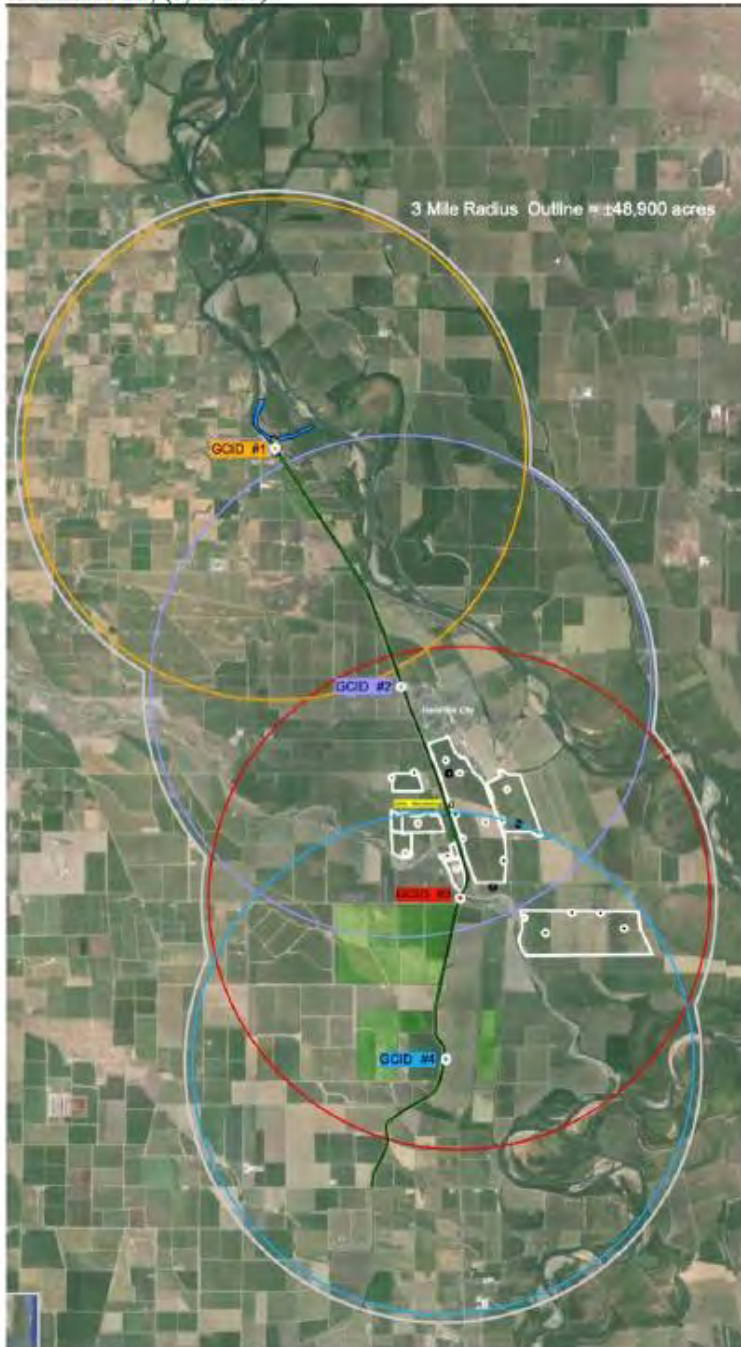
Figure 5. GCID owned production wells, and their areas of influence in the vicinity of Hamilton City (by Billiou).
